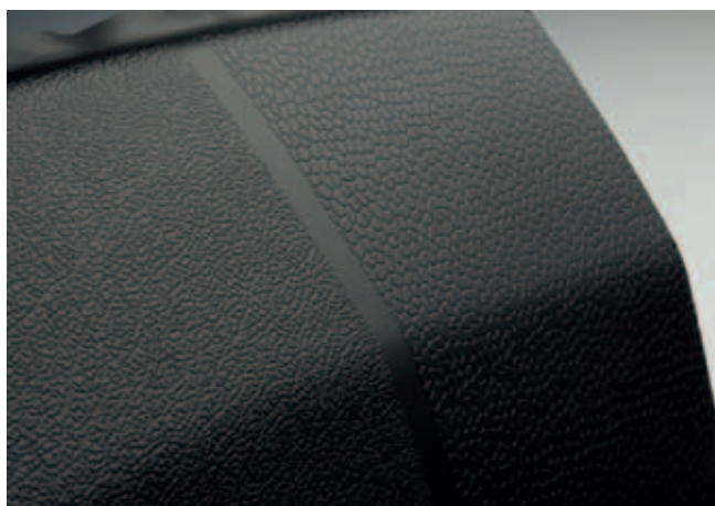
② The colour carrier is the TPO material itself, and the paint coating on it serves primarily to adjust the degree of gloss (Sample part from IAC Group and Benecke-Kaliko)
