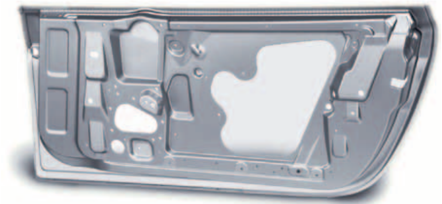
③ With a length of maximum 1281 mm, the Aston Martin door inner frames made from magnesium are of above-average size
