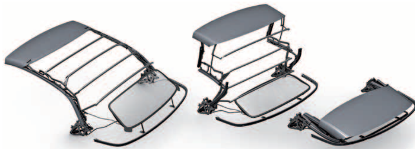
5 Movement profile of the softtop when opening and closing
