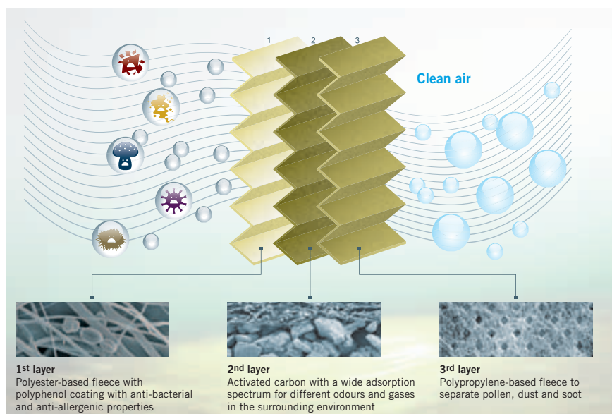
6 Effective health protection through three filter layers – the first layer consists of a polyphenol coated non-woven material
